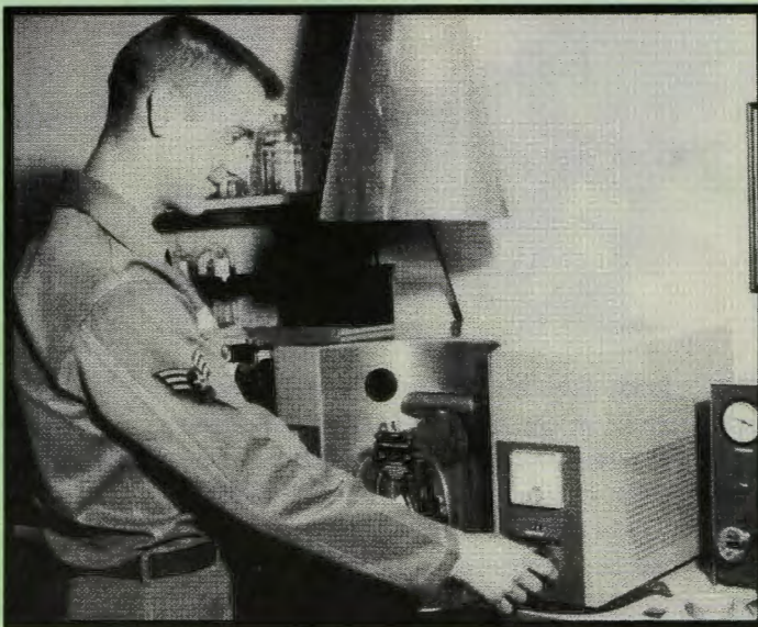
Technician takes the absorption reading of an oil sample
