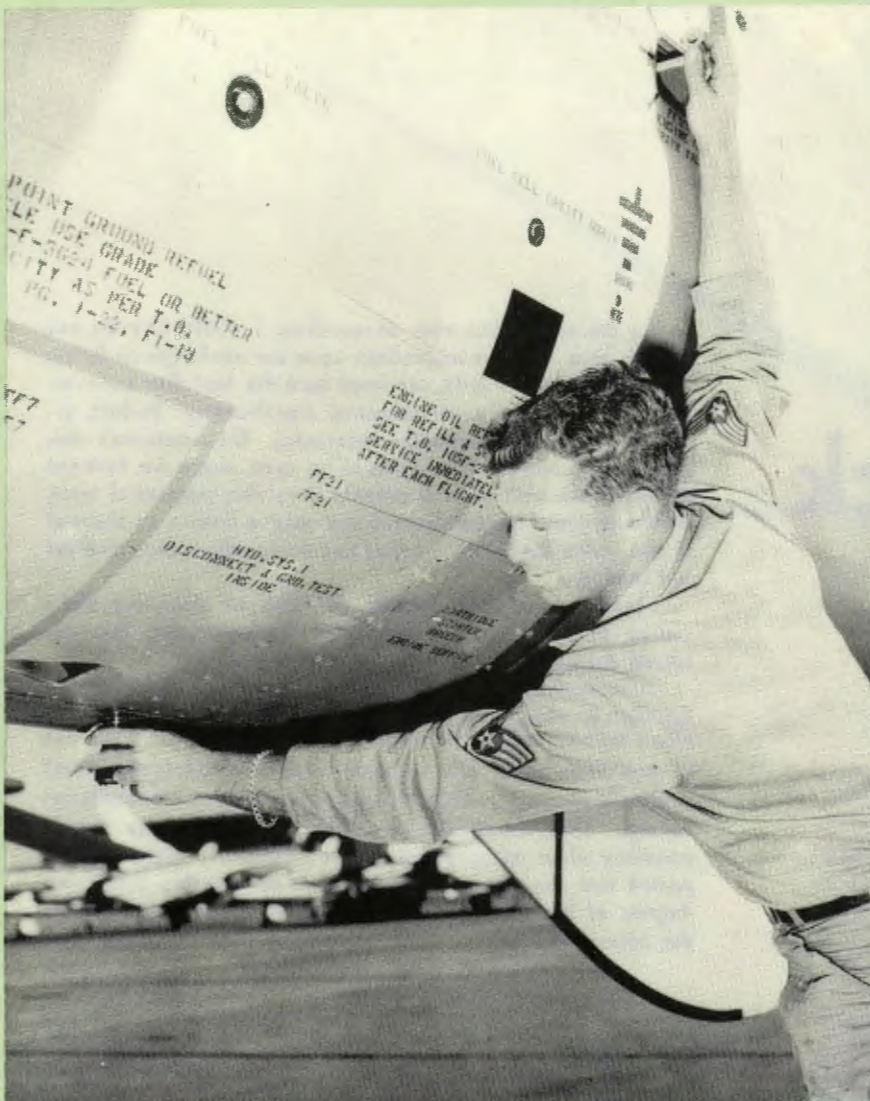
Crew chief takes an oil sample during shut down procedure
